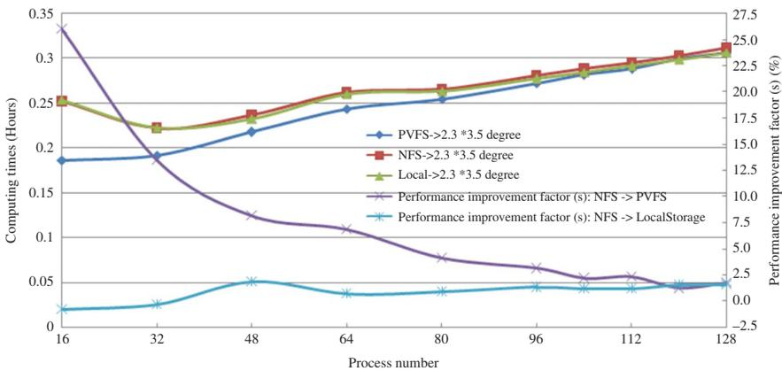
Figure 9. Using different file systems to run the NMM-dust storm model for domains  $2.3 \times 3.5$  degree in the southwest United States with 3 km resolution, for 3-hour predictions. The PVFS2 achieved a 20% performance improvement (*s*) than that of NFS.
